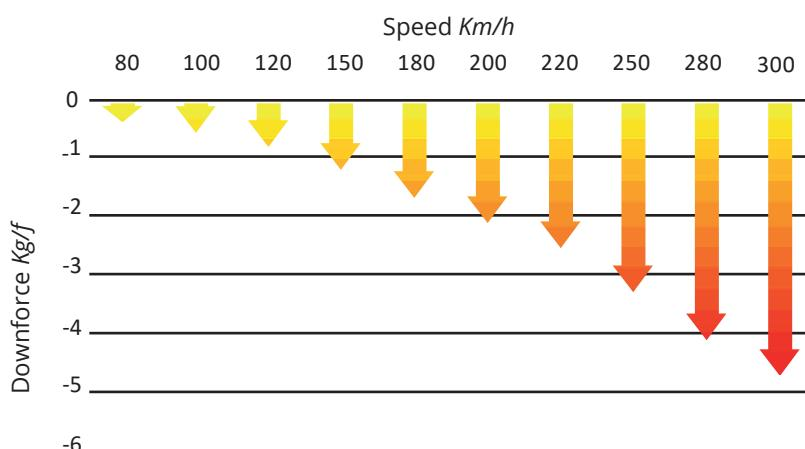
The Downforce that the spoilers generates raises potentially as the speed increases, at 200 km/h we get 2,2 Kg/f.
