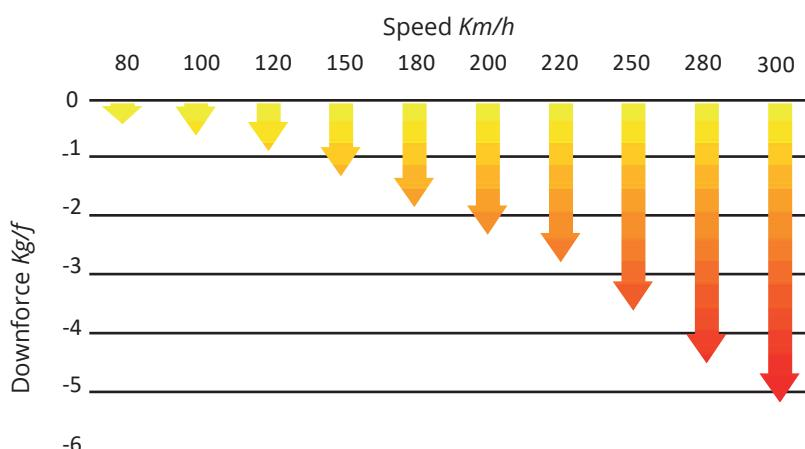
The Downforce that the spoilers generates raises potentially as the speed increases, at 300 km/h we get 5,2 Kg/f.
