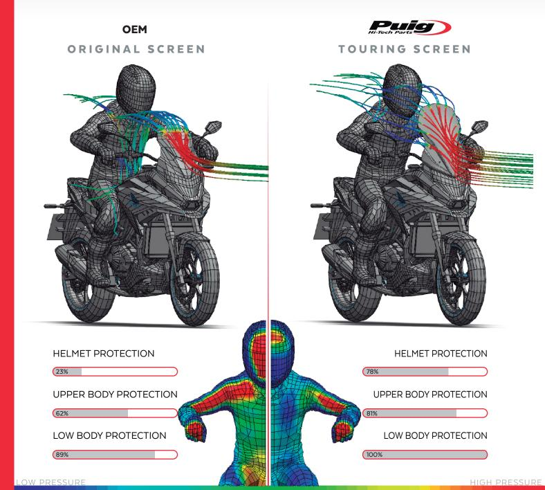
TOTAL DISSIPATED PRESSURE WITH PUIG SCREEN IS EQUIVALENT TO 5,7 Kg
